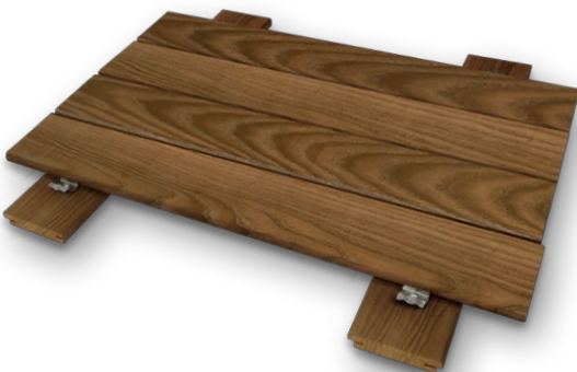
Tavole in TERMO FRASSINO spess.19/21 x largh.95 x lungh.1200/3500 mm ca. Con o senza zigrinatura antiscivolo e fresatura per clips THERMO-ASH approx. thickness 19/21 x width 95 x length 1200/3500 mm. Smooth or with non-slip ridges and clip grooves
