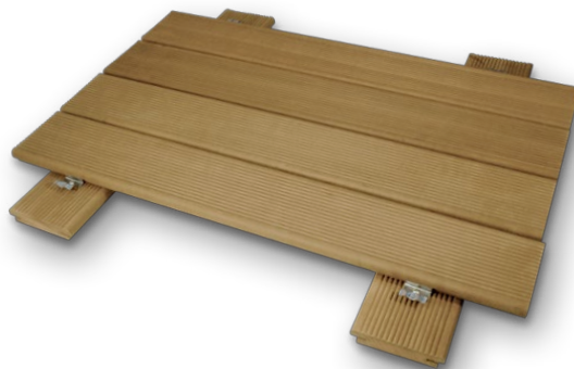
Tavole IPE' LAPACHO spess.19/21 x largh.90 x lungh.900/3000 mm. Con o senza zigrinatura antiscivolo e fresatura per clips IPE' LAPACHO BOARDS thickness 19/21 x width 90 x length 900/3000 mm. Smooth or with non-slip ridges and clip grooves
