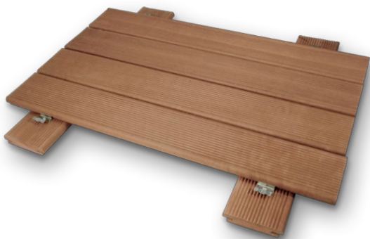
Tavole MASSARANDUBA spess.19/21 x largh.90 x lungh.900/3000 mm ca. Con o senza zigrinatura antiscivolo e fresatura per clips MASSARANDUBA approx. thickness 19/21 x width 90 x length 900/3000 mm. Smooth or with non-slip ridges and clip grooves
