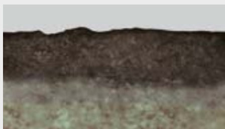
Cross-section of a nadura element with heavily reinforced wear layer directly attached to a special board°– in an electron microscope.
