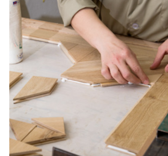
Manual assembly of the Quadrotte
