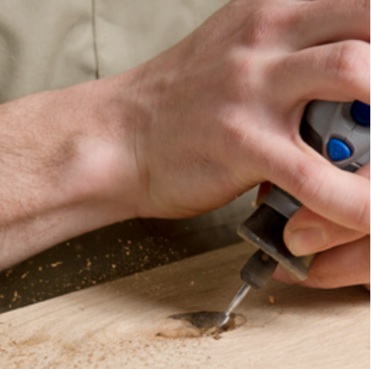
Preparation of the knots for filling
