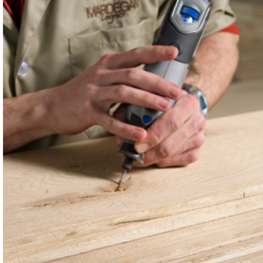
Preparation of the knots for filling
