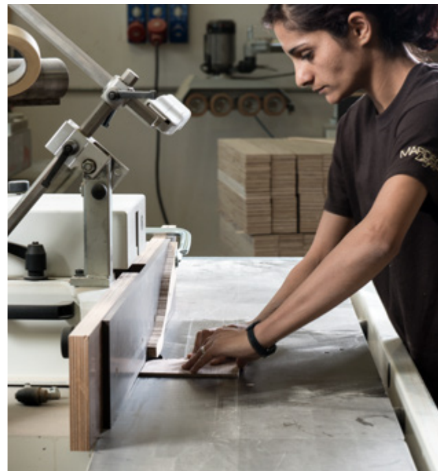
Details of the phases of manual workmanship for cutting, chamfering, and assembling the Teorema boards.
