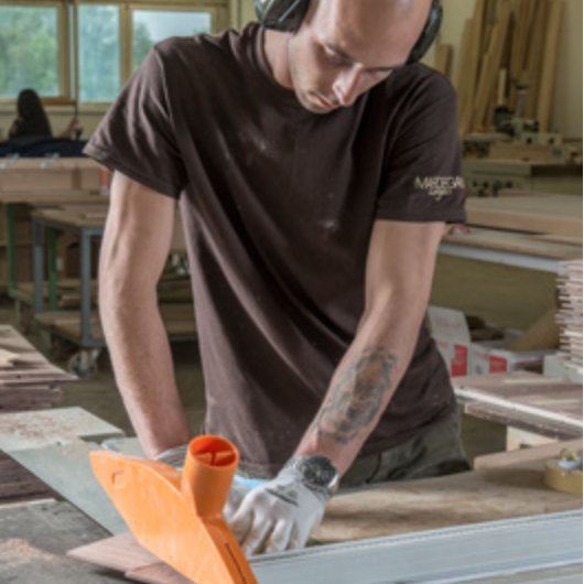
Cutting the plugs for the Teorema boards
