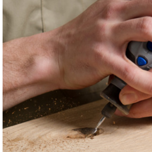
Preparation of the knots for filling
