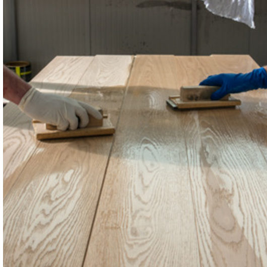
Finishing with the oil-wax treatment
