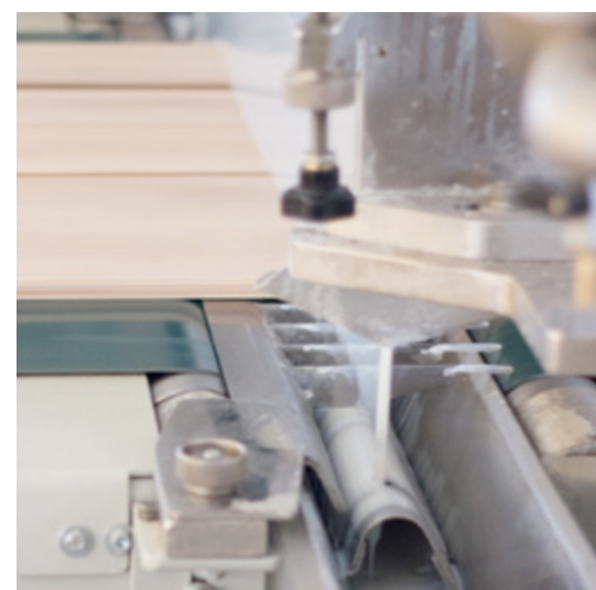
Application of water-based protective varnish
