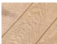
Brut de sciage Band saw marks
