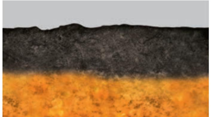
Cross-section of Nadura element with heavily reinforced wear layer directly attached to a special board, in an electron microscope.
