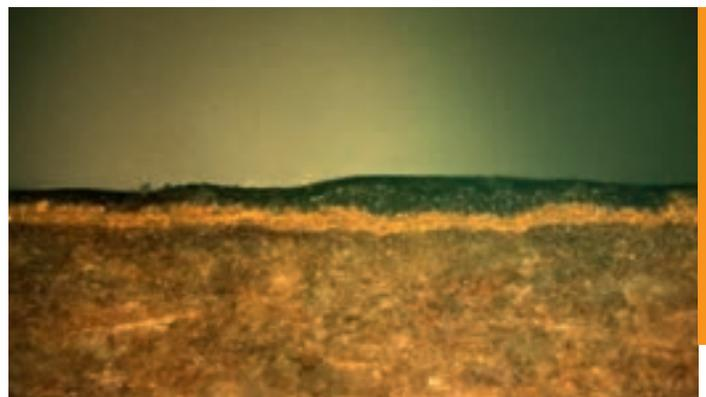
Cross-section of laminate with a wear layer made of overlay, decor paper and HDF middle layer, in an electron microscope.
