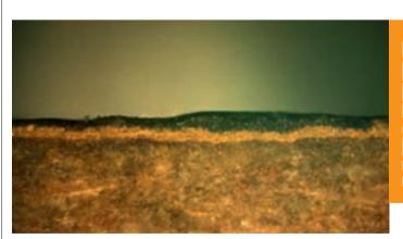
Cross-section of laminate with a wear layer made of overlay, decor paper and HDF middle layer, in an electron microscope.
