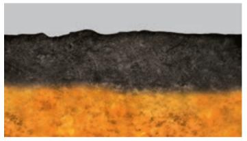
Cross-section of Nadura element with heavily reinforced wear layer directly attached to a special board, in an electron microscope.
